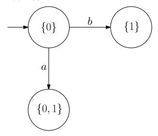
Summarizing in a different way: we start in a situation where the NFA is in state 0 in all possible universes (represented by state  $\{0\}$ ). In all these universes, if the NFA reads an a, it can be in either state 0 or 1 in any possible universe (represented by state  $\{0,1\}$ ). On the other hand, in all these universes, if the NFA reads a b, it ends up in state 1 in all possible universes (represented by state  $\{1\}$ ).
