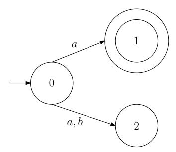
In this case, there are two arrows labelled with a coming out of state 0 – one to state 1, and one to state 2. There are also a lot of arrows missing... Can you point out where?
